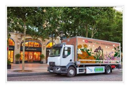
As part of its research into goods transport based on sustainable development, Renault Trucks and Guerlain are currently testing an experimental all-electric vehicle operated by Speed Distribution Logistique. This 16 t vehicle will be delivering supplies to Maison de Parfums & Cosmétiques boutiques in Paris over the next two years. It generates no polluting emissions or noise nuisance and will be tested on regular, demanding delivery rounds of over 200 km.
